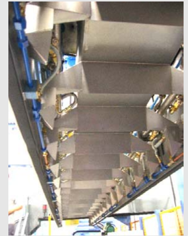
Fig. 6) Adaptation of sprayers according to the profile type.
